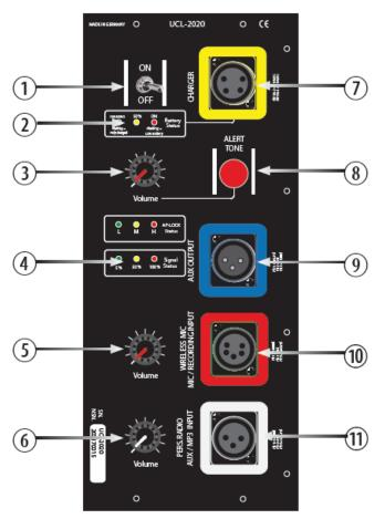
① ON / OFF Switch • ②ON / OFF Indicator / Bat.-Status • ③ Siren/Alarm Volume • ④ Signal / Output Status • ⑤ Personal Radio/Mic-AdHoc-Recording Volume • ⑥ External Wireless/Aux/ MP3 Volume •
