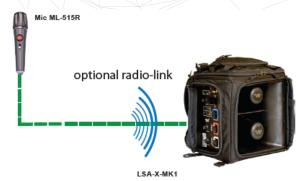
Direct cable connection or radio link
